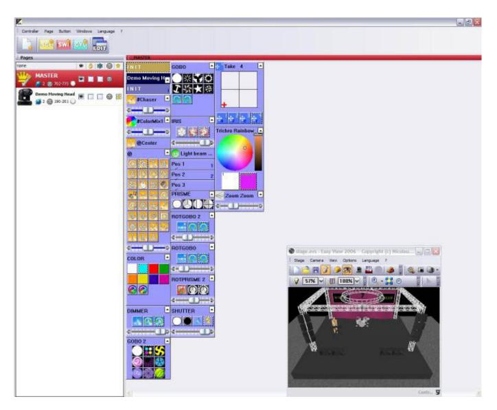
The Sunlite software will display 1 button for every function that the lighting fixture can perform. There will be 1 button on the screen for every color, gobo, macro, prism effect, etc.
