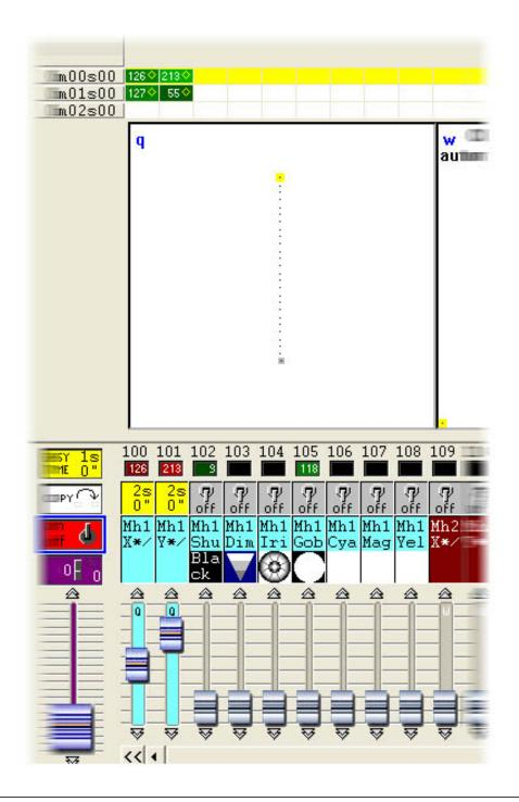
Once we have made this, we can copy the "PAN&TILT" channels and paste to one fixture. The "Copy/Paste" window appears and we must select "Advanced" to access the phasing function. After having selected "Phasing (only with EasyTime or EasyStep channels)", you must specify the type of phasing:
