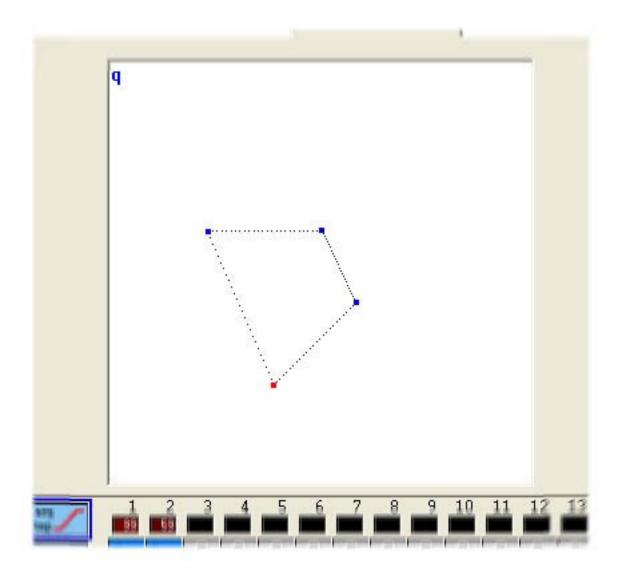
Each corner in the picture represents the X-Y position in each step. These can be moved individually with the mouse. Steps with fade in between show dotted lines in between the corners in the shape area. Steps can be selected by clicking on the corresponding point (white area) or directly from the step list at the top.
