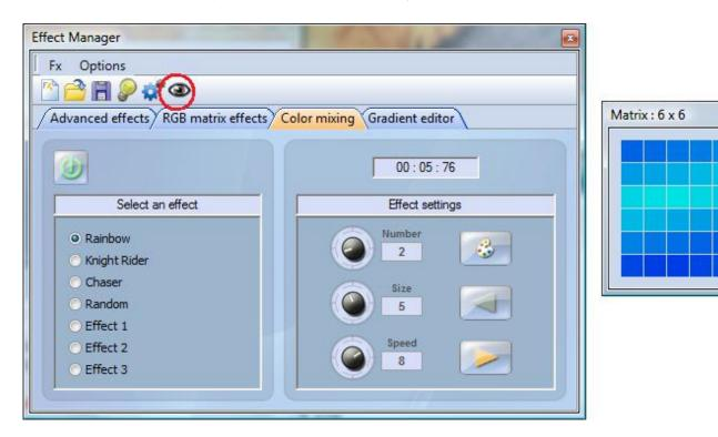
You can vary the size, speed and direction of the effect as well as changing the colours used by clicking the pallet icon. You can also change the number of colours used. Remember to click generate before closing the effect manager.
