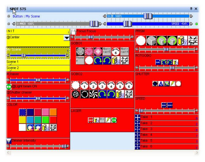
You can see the new toolbar appear above the buttons on the selected page. The three faders on this toolbar will control whatever button is selected (a SELECTED button is not necessarily the same as an ACTIVATED button, you can SELECT without ACTIVATE by left-clicking with the mouse).
