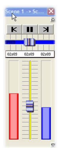
Please keep in mind that the FADE function is not available on channels which have been programmed with the ON/OFF mode. This is very useful to make some channels fading or not in a scene. Imagine you want to fade from one position to another one with your fixtures but you want to change the gobo without fading in the same scene. The gobo channel must be programmed with the ON/OFF mode, or the FADE function (Page Settings window) must be disable on this channel.
