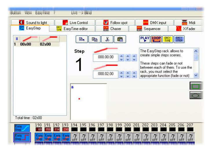
You can change the properties for each channel manually, if you want. Simply select any of the buttons on the bottom left (2 EasySteps, 1 ON/OFF, 1 Dimmer), and then click at the top of each channel. For the moment, it is best if you leave all channels as EasyStep channels.
